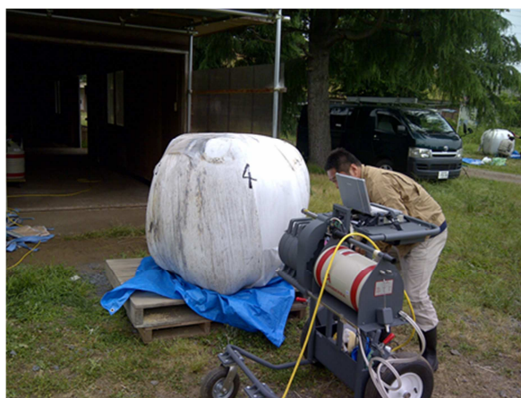
Fig. 5. The ISOCS in-situ Ge measurement
