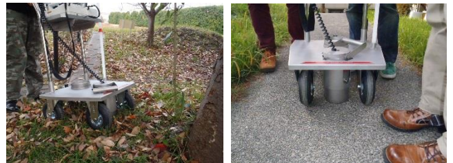
Photo.3-1, 3-2 The present condition of measurement. In the measurement on concrete, the distance of the ground and a survey meter is kept exact. It can measure in measurement of soil, without shaking.
