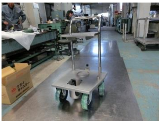
Photo.2 The measurement carry. Measurement carry puts a lead shield and is movable. There are four tires and there is little vibration.
