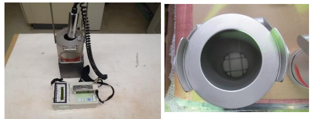
Photo.1-1, 1-2 The leaden shield for the survey meter. The leaden shield with a thickness of 3cm covers 90% of \gamma -ray.
